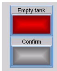
Figure 23: Empty tank command has to be confirmed by a second button
