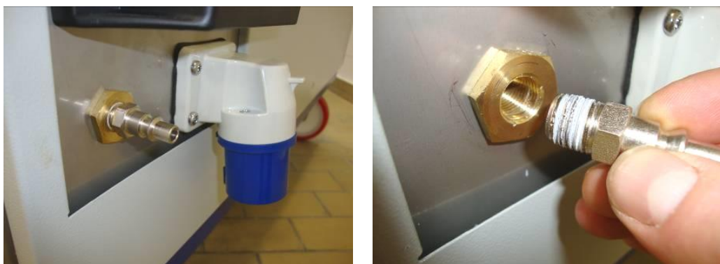
Figure 14: Changeable ¼" pneumatic plug
