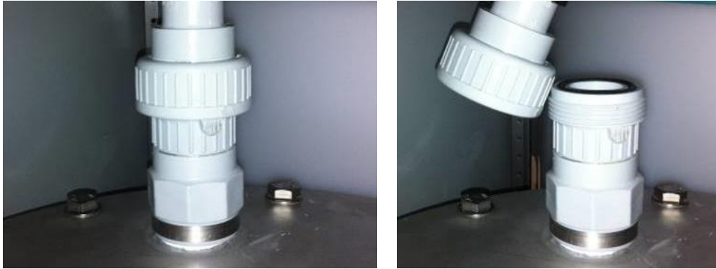
Figure 36: Disconnecting top hose of the resin tank
