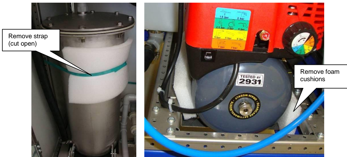
Figure 6: Remove the transport securing devices
